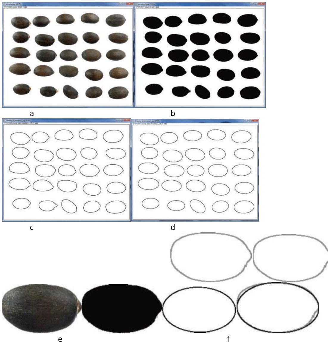
Figure : Digital processing of seed images. (a) Images corresponding to 25 seeds. (b) Binary images (black and white) of the seeds obtained by the figure. (c) Silhouettes of seed images. (d) Ellipses adjusted to each seed image (fitted ellipses are given by the program Image J). (e) A seed with its image after segmentation and the silhouettes of the image (top) and the adjusted ellipse. (f)
